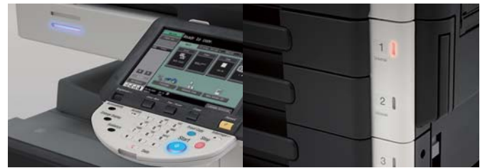
Status lamp shows machine condition.
